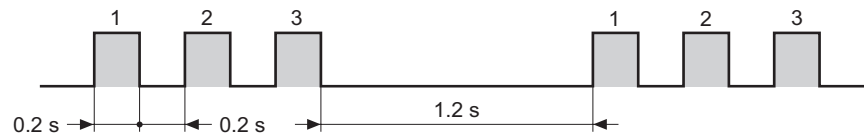
Figure 6-5 Blink Pattern of ALARM LED
