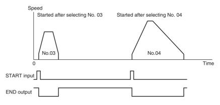
An END signal is output when the positioning operation is complete.
