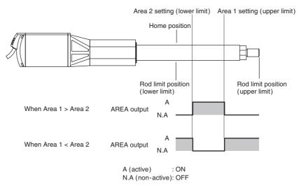
When Area 1 = Area 2, the AREA output becomes active only when the slider/cylinder is at the set position.
