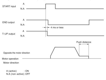
Figure 4-28 T-UP Output (pushed condition not achieved)
