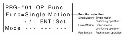
To start a positioning operation, select the number in which the operation data you wish to execute is set, using the input M0 to M5. If a number between 01 and 63 is selected, it means either the single-motion positioning operation or linked-motion positioning operation has been selected.
