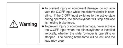
When the C.OFF input is activated, the motor output current will be cut off (the slider/cylinder will lose its holding brake force).
