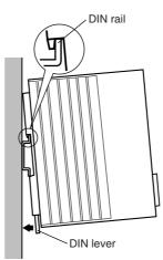
Secure the controller using an end plate.
